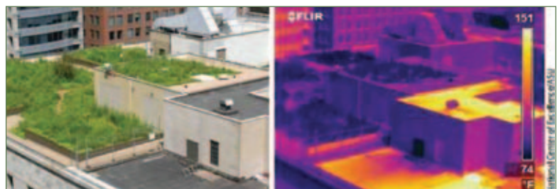
On a typical day, the Chicago City hall green roof measures 80°F (40°C) cooler than the neighboring conventional roof.
